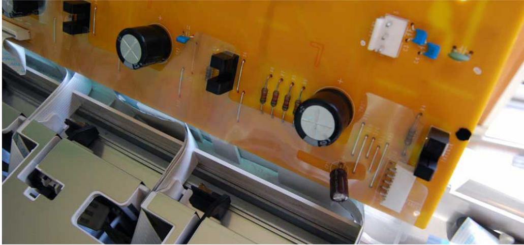
Using scissors, make some cuts in the acetate to enable its easy removal. There is no need to remove anything else from the pcb.
